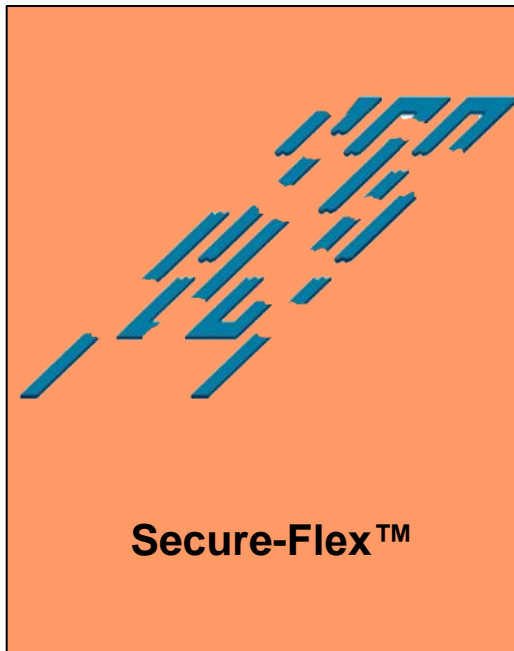
Device disabled - Conductors broken
