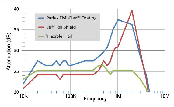
Testing performed by independent third party certified testing facility using standard Parlex cables treated with Parlex EMI-Flex™ coating and competitive offerings (June 2012).
