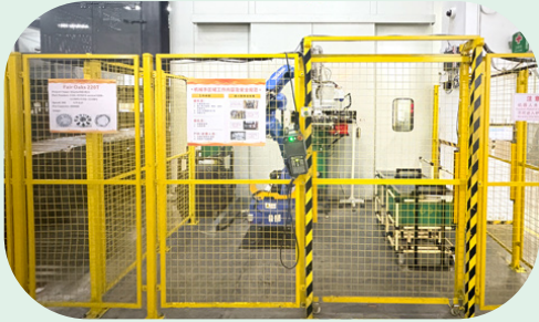
AI-enabled electronic fence in our Jiangmen, China production site to enhance robotic arm safety.
